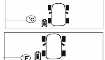
After the Temperature type has been selected Press the SET BUTTON again to enter the High Pressure setting mode. It will Beep and flash the High Pressure alarm setting. This can be increased or decreased by pressing the LEFT or RIGHT BUTTON
