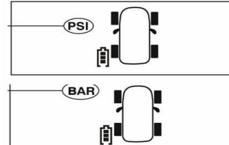
After PSI or BAR has been selected Press the SET BUTTON again to enter the Temperature setting mode. It will Beep and flash the Temperature setting. This can be switched between C & F by pressing the LEFT or RIGHT BUTTON
